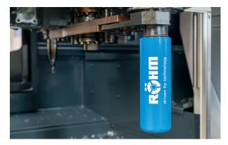
After the lubrication process, Lubritool<sup>®</sup> is sent back to the tool magazine and remains there until the next lubrication cycle.
