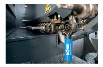
Lubritool<sup>®</sup> is located in the tool magazine. Whenever the machine control notifies that a lubrication process is necessary, Lubritool<sup>®</sup> will be sent up into the spindle.
