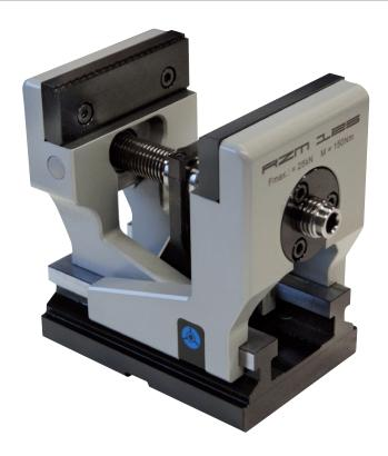
The **RZM** centric clamping vice is ideal for 5-axis processing centres. Without any additional substructures or special jaws, the centric clamping unit holds the workpiece securely – with a minimum interference contour.
