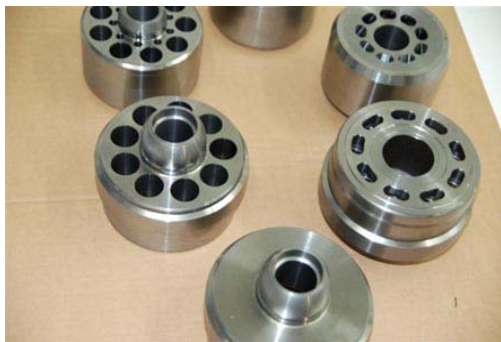
Image no. 15-03 RM_MIK-Teile2.jpg Workpieces made of aluminium and GGG 60 spheroidal cast iron are guided through the system securely with a single set-up.
