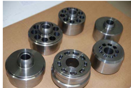
Image no. 15-02 RM_MIK-Teile.jpg In one set-up, completely machined parts for the hydraulic drive in heavy building machinery.
