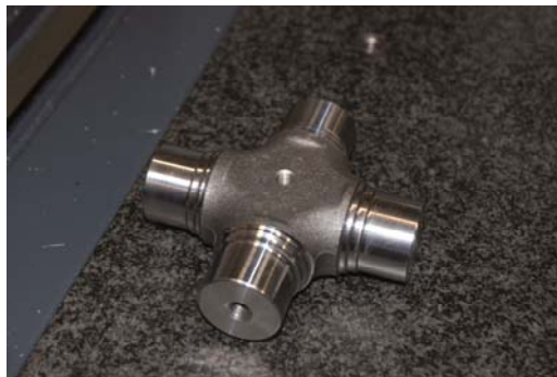
Wanxiang makes as many as 60 million of these cardan joints a year for the automotive industry.
