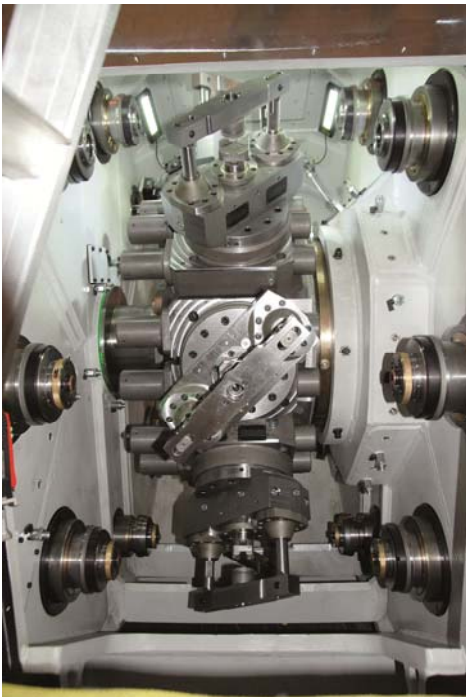
A total of eight units consisting of clamping tools and rotary machine table are incorporated in Witzig & Frank's rotary transfer machine, making it possible for the workpiece to be processed at eight stations with different manufacturing technologies.
