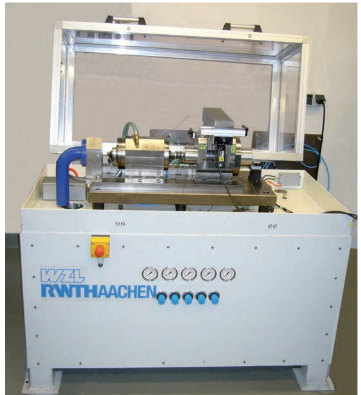
The test bench for tool clamping systems during testing at RÖHM Sontheim.
