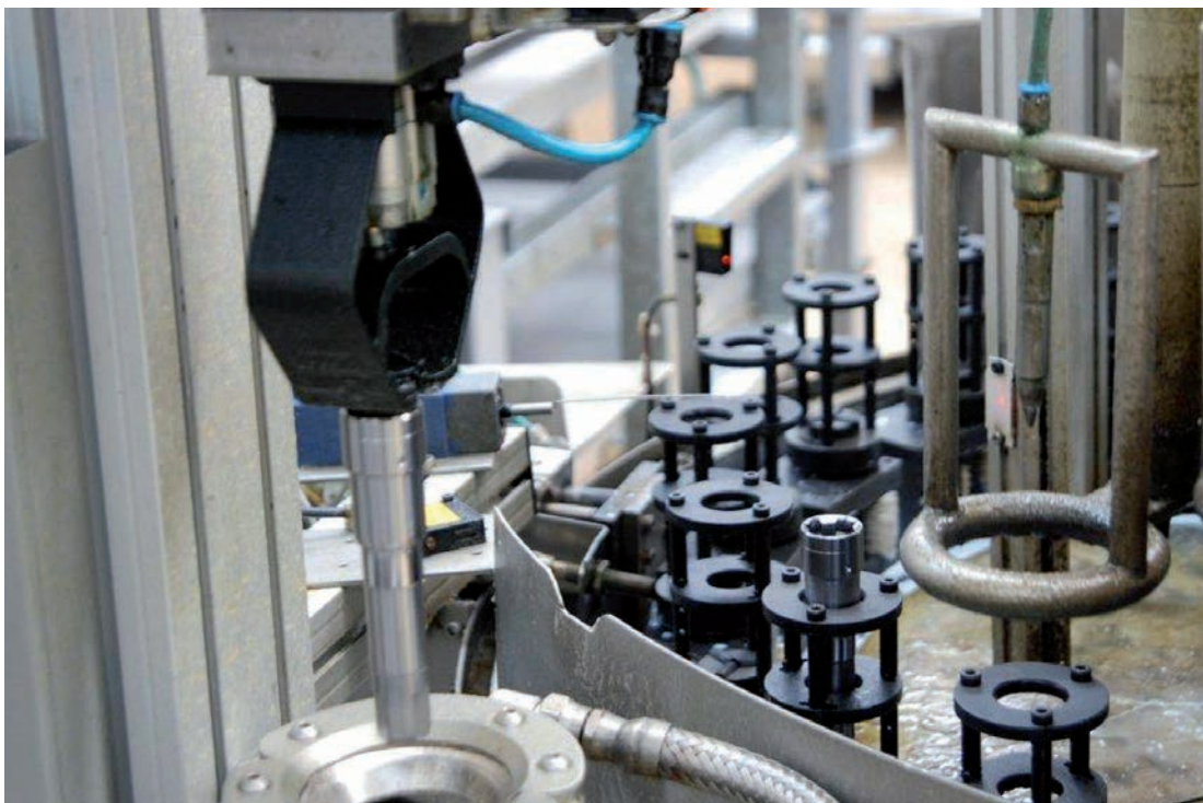
Discussions with the customer resulted in the solution – using a piston which provides additional clamping strength to the mandrel.
