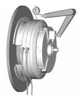
When dismantling the chuck from the spindle nose, the clearance console is not dismantled from the distributor ring and is just loosened from the spindle box.
